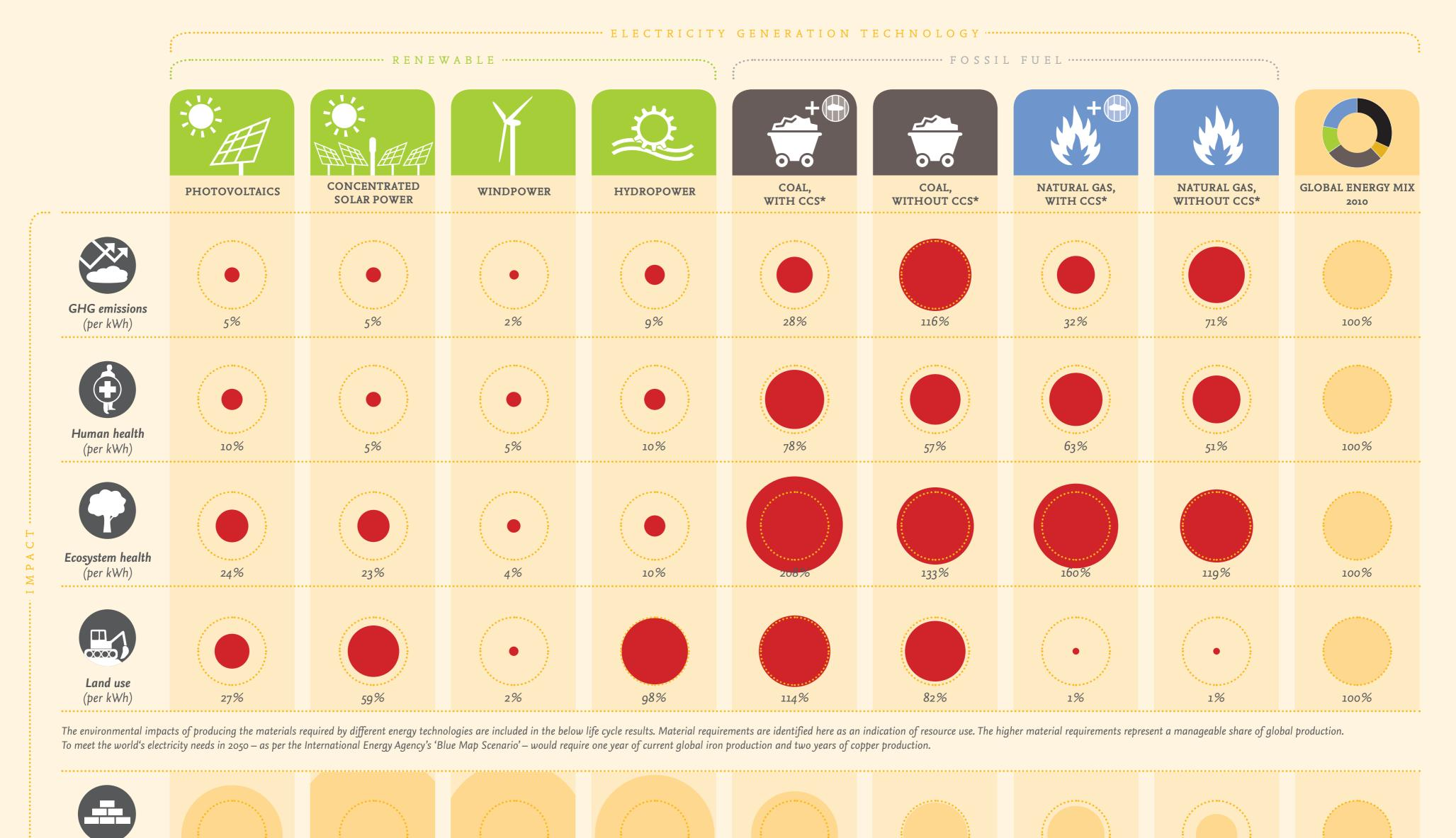
\* Carbon capture storage (CCS) technology entails the capture of CO2 from large anthropogenic sources, transport of the CO2 to an underground storage reservoir and long-term isolation from the atmosphere.
