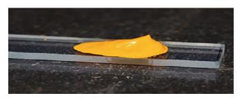
**Solar paint would transform almost any surface into a cheap solar panel.** It could work on rooftops, walls, cars, cell phones, and more. It involves applying a conductive layer, then a white base layer, and finally a light-sensitive dye on top—this is what generates the electricity—and applying heat to cure the paint. In theory, it would be as straightforward as painting a wall in your house. Source: NDnano, University of Notre Dame
